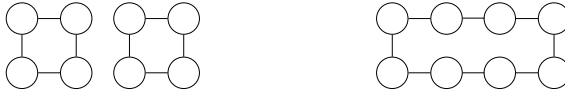
Figure 7.1: Two graphs that are not distinguishable by 1-WL or most GNNs. The left graph consists of two cycles of length 4. The right graph consists of one cycle of length 8. In every GNN message-passing step, there are 8 nodes; no node has any features and receives a message from exactly 2 featureless nodes. No node can gain information to differentiate between the two graphs.
