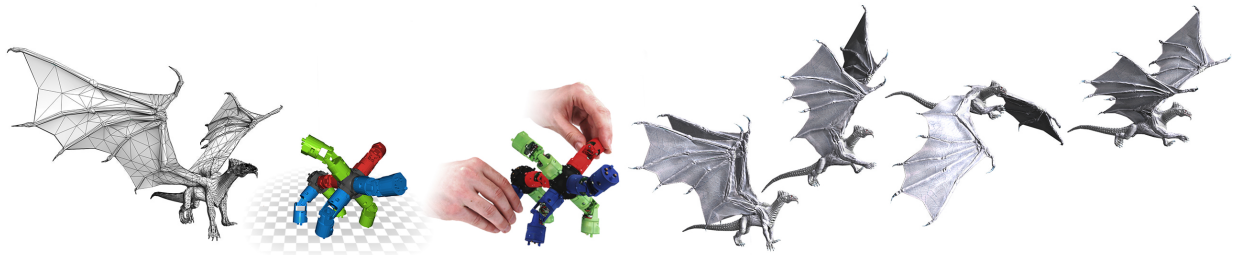
Figure 3.1: Left to right: Taking a rigged 3D character with many degrees of freedom as input, we propose a method to automatically compute assembly instructions for a modular tangible controller, consisting only of a small set of joints. A novel hardware joint parametrization provides a user-experience akin to inverse kinematics. After assembly the device is bound to the rig and enables animators to traverse a large space of poses via fluid manipulations. Here we control 110 bones in the dragon character with only 8 physical joints and 2 splitters. Detailed pose nuances are preserved by a real time pose interpolation strategy.
