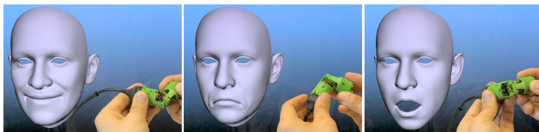
Figure 3.16: Controlling a face blendshape rig with a single joint. We manually map the angles of the joint such that they semantically match the facial expressions (i.e., a \vee shape for smiling, a \wedge for frowning, and twist opens the mouth).
