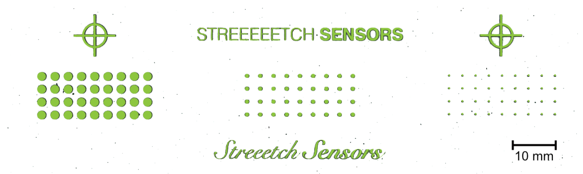
Figure 4.8: To demonstrate the alignment quality of our fabrication method, we produced a test pattern with two identical conductive (black) layers. The fabricated pattern was scanned with a flatbed scanner. The scan is overlaid with the digital design (green). Wherever the alignment is perfect, only the green layer is visible.
