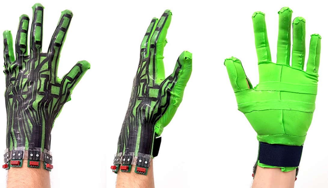
Figure 5.2: Our glove consists of a full soft composite of a stretchable capacitive silicone sensor array and a thin custom textile glove (green).
